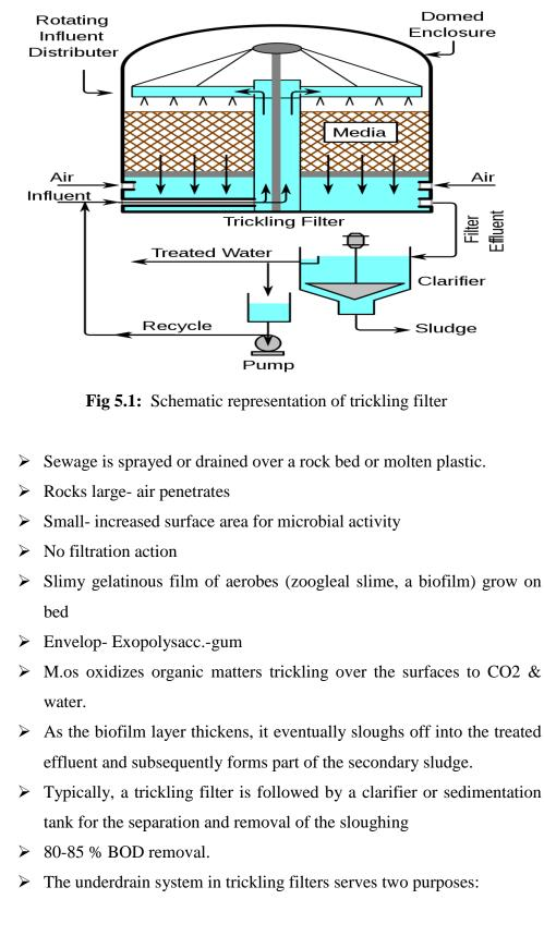
(a) To carry the wastewater passing through the filter and the sloughed solids from the filter to the final clarification process, and
