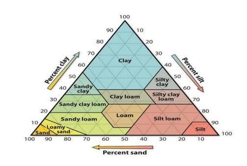
Fig 8.2: The textural triangle of soil according to the texture the soil properties may differ. (Source: Soil science society of America)
