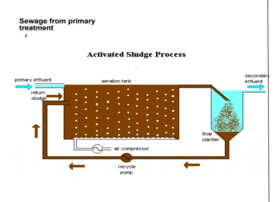
Fig 5.2: Schematic representation of Activated sludge process
